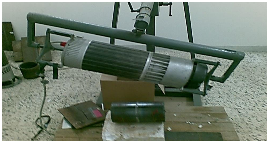
Figure 7. X-ray machine and imaging angle at 45°
