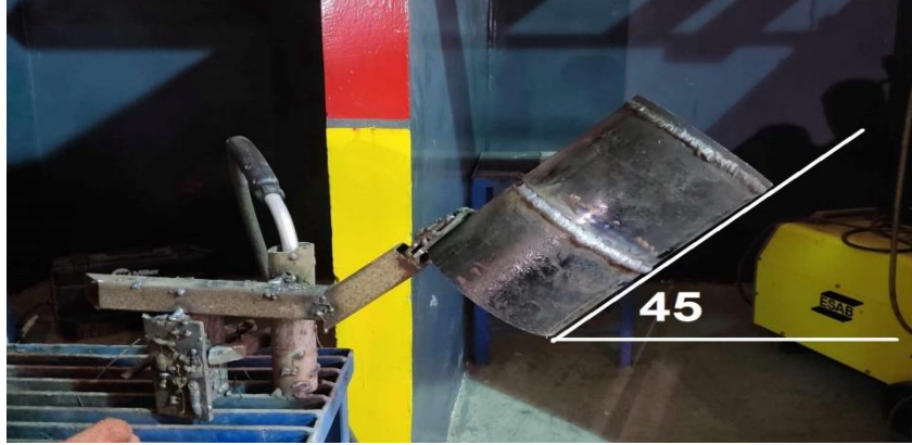
Figure 6. 6G welding position
